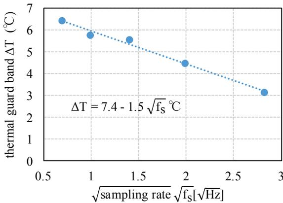
Fig. 6. Thermal guard band variation as a function of the sampling rate
