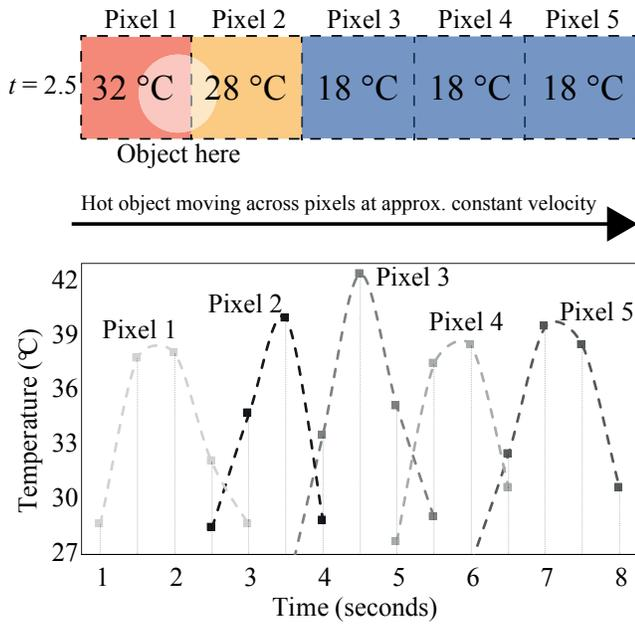
Fig. 4. Temperature plot a single line of pixels in the MLX90620's thermal array as a hot object moves across them at a constant velocity
