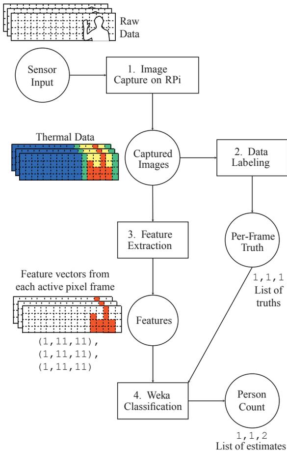
Fig. 3. Process flow diagram for turning raw sensor input into occupancy estimates
