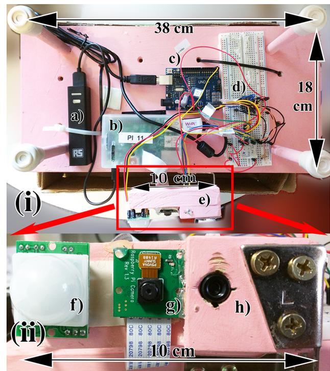
Fig. 1. (i) top view layout of the circuit containing a) Battery pack, b) Raspberry Pi, c) Arduino, d) Level-shifting circuitry, e) Movable sensor mount, f) PIR, g) visible camera, h) MLX90620; (ii) front expanded view of the 3 sensors
