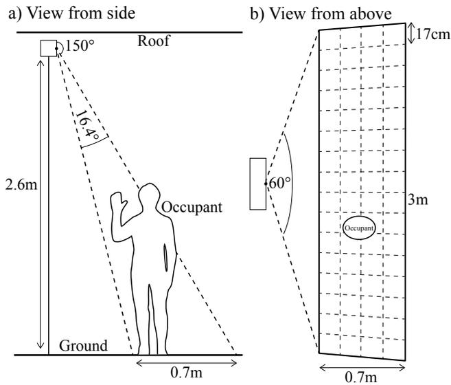
Fig. 2. Physical arrangement of the classifier experiment including (a) side view showing test rig in Fig. 1 mounted at ceiling height, (b) physical extent of the mapped area [20]
