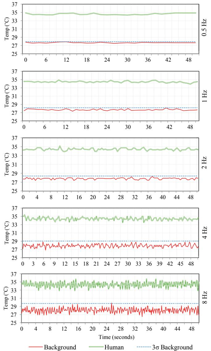
Fig. 5. Plot of occupant and background sensor noise at sampling speeds 0.5 Hz – 8 Hz
